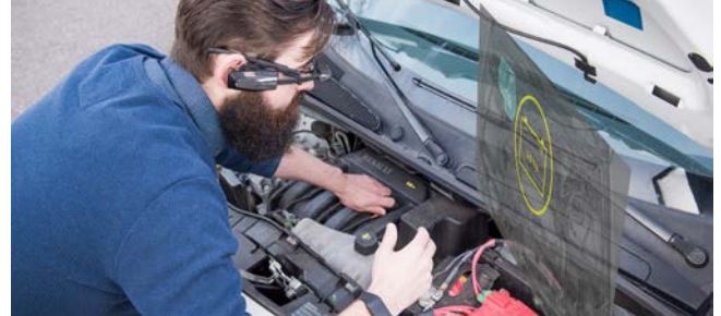
The manual for a vehicle's maintenance work can be used by gesture control.
